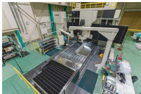
超精密静圧門型複合加工機 Super precision oil static double column complex process grinder
